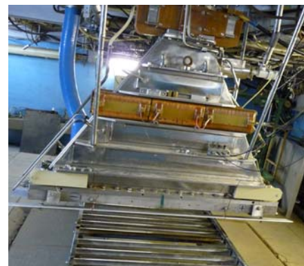
Fig.7 ILU-10 beam scanning horn and roller conveyor.
