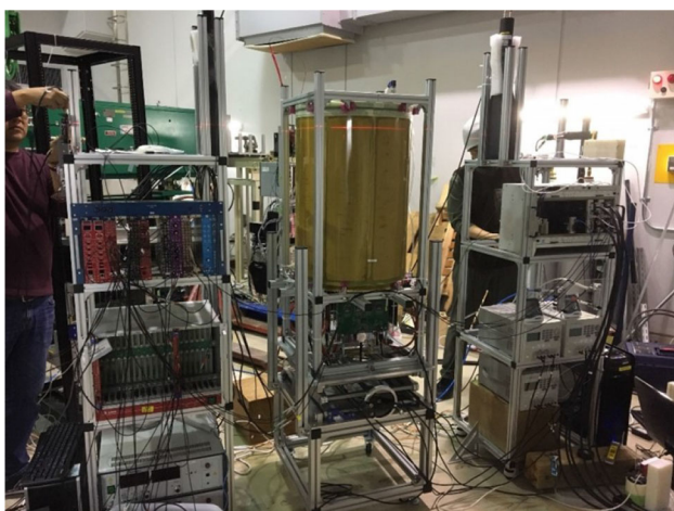
Fig. 3 (Color online) Picture of the experimental setup at the ELPH. The prototype TPC is installed vertically in the center. The TPC can move vertically to change the beam injection position in it. The trigger counters are installed at the entrance and exit of the beam in TPC, and the readout electronics can be seen in the adjacent racks
