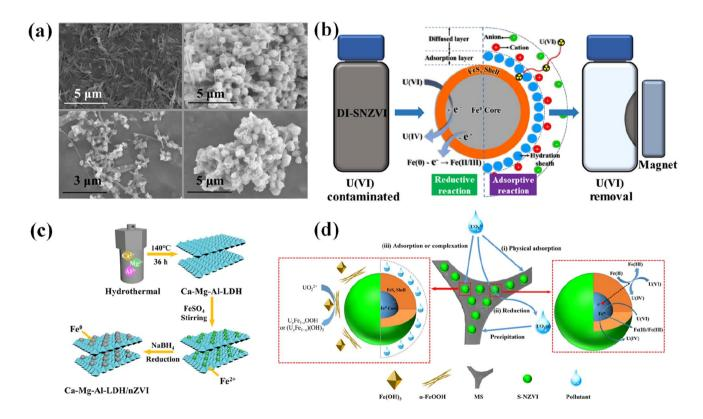
**Fig.4** (Color online) **a** Scanning electron microscopy images of  $Na_2V_6O_{16}$ -2H<sub>2</sub>O nanobelts before and after the extraction of U(VI) at different concentrations [55]; **b** schematic diagram of U(VI) uptake from wastewater by adsorptive and reductive processes using sulfur-
