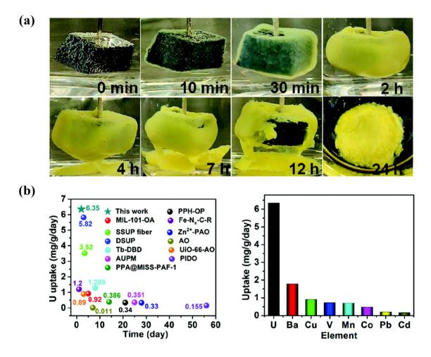
**Fig. 3** (Color online) **a** Photographs of Fe–N<sub>x</sub>–C–R electrode in uranium-spiked seawater during electrocatalytic extraction [53]; **b** U(VI) extraction by In–N<sub>x</sub>–C–R and other materials (left); extraction selectivity of U(VI) by In–N<sub>x</sub>–C–R from natural seawater (right) [54]
