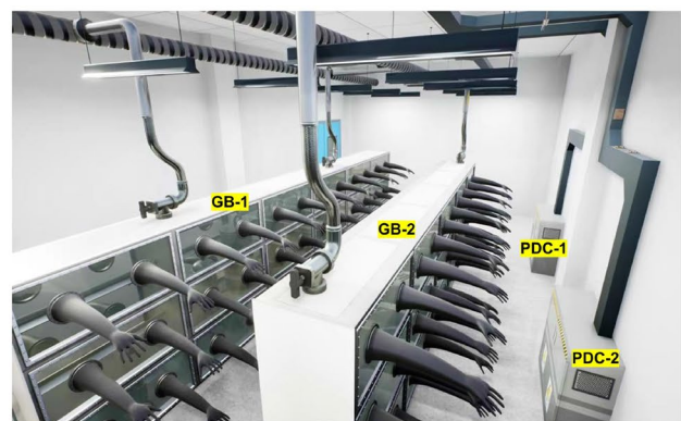
Fig. 1 (Color online) TEP process room. a Schematic of TEP process room from top view; b 3D virtual geometric scene built by out tritium technology team
