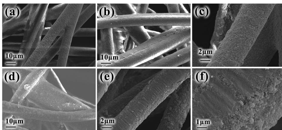
**Fig. 4** (Color online) Images of pristine **a** PP/PE SNW, **b** P-HBP-AO, and **c** P-HBP-AO-U after uranium adsorption. **d** EDS mapping image of uranium.
