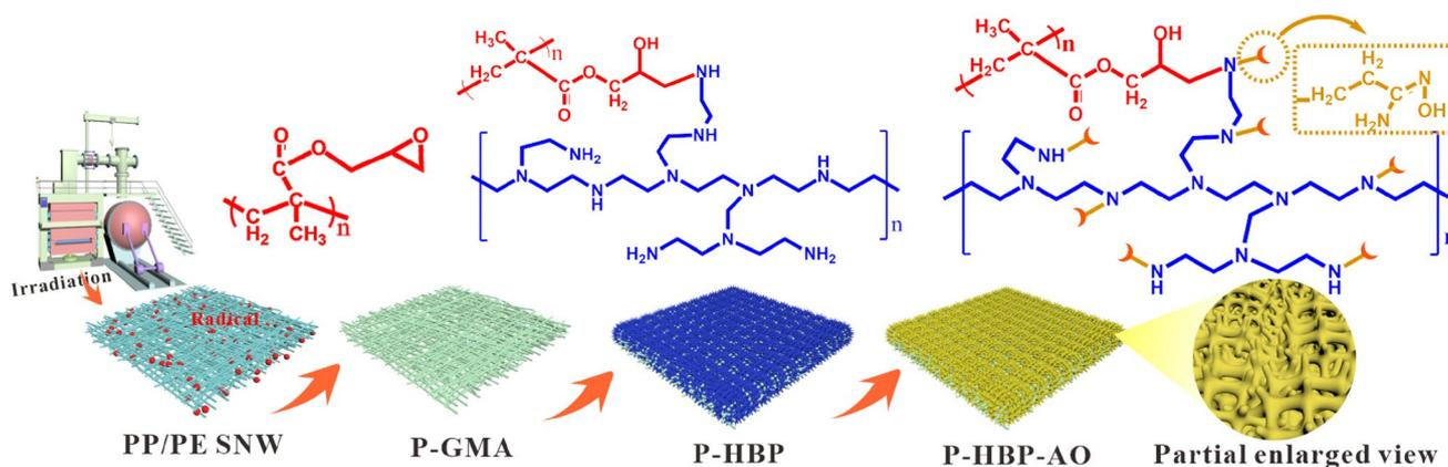
**Scheme 1** (Color online) Schematic of the fabrication process and chemical structure of P-HBP-AO
