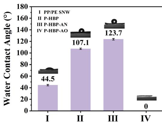
**Fig. 6** (Color online) Water contact angle for PP/PE SNW, P-HBP, P-HBP-AN, and P-HBP-AO
