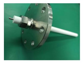
Fig. 8 (Color online) Image of the high-voltage feedthrough
