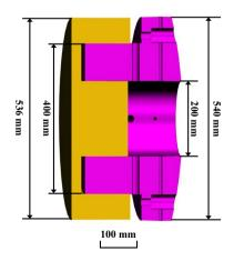
Fig. 5 (Color online) Cross-sectional view of the cooling base and tube
