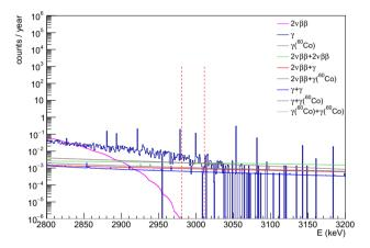
**Fig. 14** (Color online) Energy spectra for various single-event and pile-up backgrounds of the  $N\nu DEx-100$  experiment with natural  $SeF_6$  gas without further suppression using event topology information
