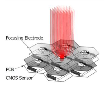
Fig. 9 (Color online) Topmetal-S sensors tiled in a hexagonal pattern to form a charge readout plane without gas gain
