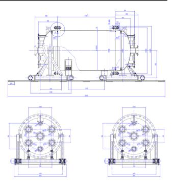
Fig. 2 Design of the pressure chamber
