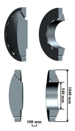
Fig. 6 Cross-sectional view of the POM fillers
