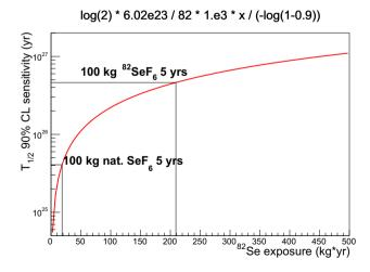
Fig. 16 Estimated  $N\nu DEx-100$  experiment sensitivity as a function of exposure
