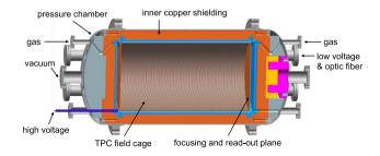
Fig. 1 (Color online) Schematic design of the main part of the  $N\nu$  DEx-100 experiment
