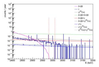
**Fig. 15** (Color online) Energy spectra for various single-event and pile-up backgrounds of the N $\nu$ DEx-100 experiment with enriched <sup>82</sup> SeF<sub>6</sub> gas without further suppression using event topology information
