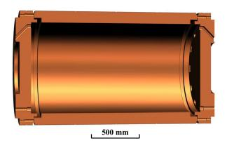
Fig. 4 (Color online) Cross-sectional view of the designed inner copper shielding
