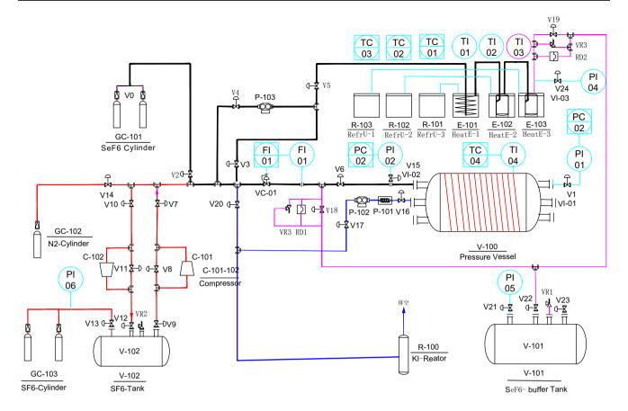
Fig. 13 Schematic of the  $N\nu DEx$  gas system
