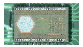
Fig. 10 (Color online) Photograph of the Topmetal-S sensor chip
